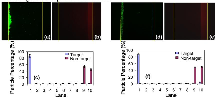
Figure 4. Distribution of target and non-target particle across the channel width at the exit of the separator. The target vs. non-target particles ratio is 1:1 in (a)-(c) and 1:10 in (d)-(f). (a) and (d) Fluorescent images of target particles. (b) and (e): Fluorescent image of non-target particles. (c) and (f): Distribution of target and non-target particles across the channel width.
