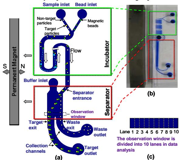
Figure 1. Integrated incubation and separation microchip. (a) Device design schematic and operating principle. (b) Image of a fabricated chip. (c) Lane division at the observation window to facilitate characterization.
