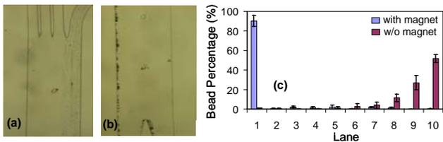
Figure 3. Separator fractionation capacity: images at (a) the inlet (b) and exit of the separator. (c) Distribution of magnetic beads at the separator exit.
